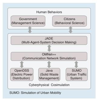
Figure 20. An MAS-based simulation platform for smart cities.
