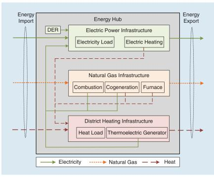
Figure 18. An energy hub configuration.
