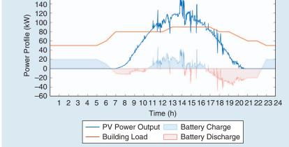
Figure 13. The power generation and consumption of the Keating nanogrid.
